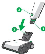
1. Connect the attachment socket (1) of the cordless vacuum cleaner to the pivot on the electric brush (2)
