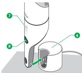
1. Ensure that the handheld vacuum cleaner is switched off before every charge.
