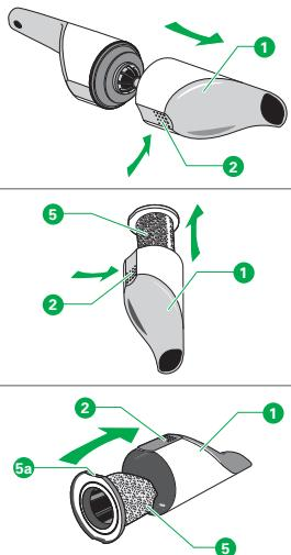
1. Press the release key (2) and remove the dust chamber from the device.
