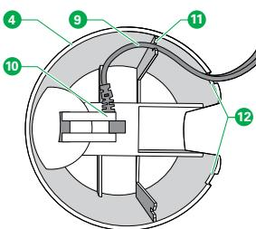
1. Plug the mains cable (9) into the designated charging socket (10) on the underside of the charging unit (4).
