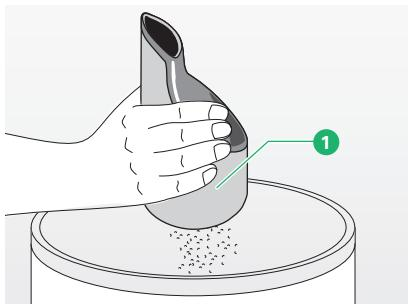
Fig. 4.10 Emptying the dust chamber
